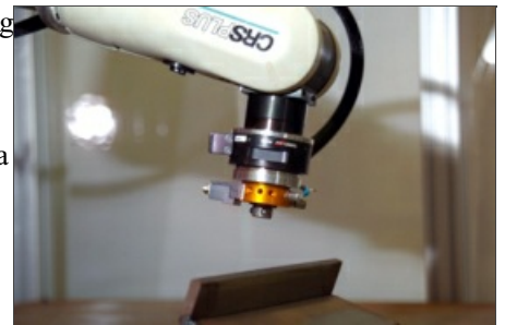
A sensor transmits force feedback from the tip of the robot's arm to a video game controller held by the user.
