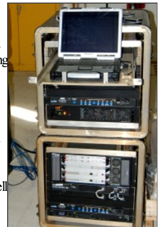
A commercial device called the Qualcomm Deployable Base Station can create an independent cell phone network.
