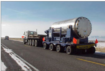
Following rail delivery to INL's Central Facilities Area, TMI core debris moved by truck and trailer to specialized examination facilities at Test Area North, 27 miles away.
