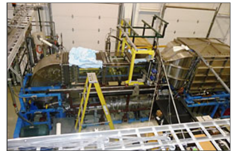
MIR is a 27-foot-long recirculating bath that can pump through 3,000 gallons of mineral oil.
